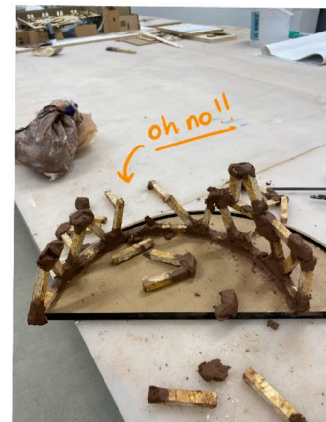
The clay was too brittle to hold the structure so the dome collapsed and a new strategy was thought of
