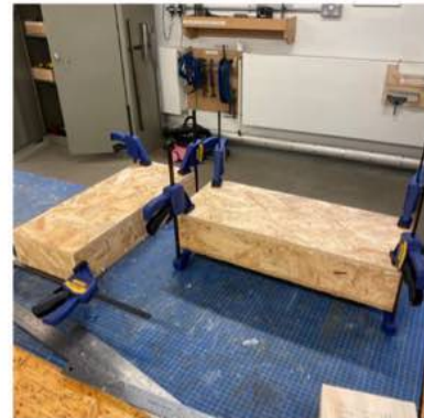
1 Making hempcrete blocks
