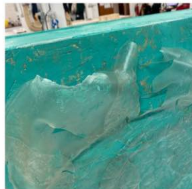
8 After drying the model cracked
