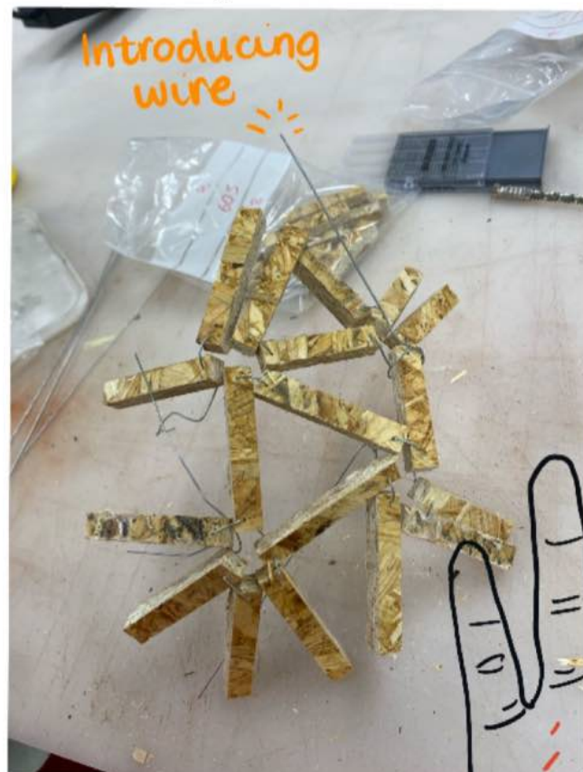
Starting to use wire to make the connections
