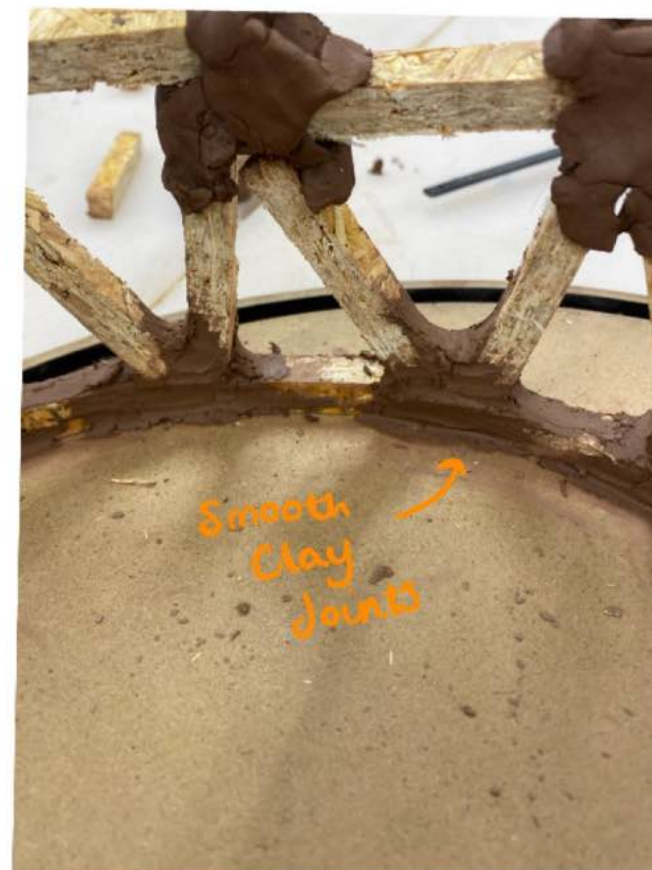
Using clay instead of adhesive to join the structure and smooth the connection
